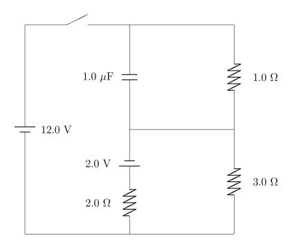
(a) Find the currents through all the resistors *immediately after* the switch is closed, before the capacitor has any time to charge up at all.
