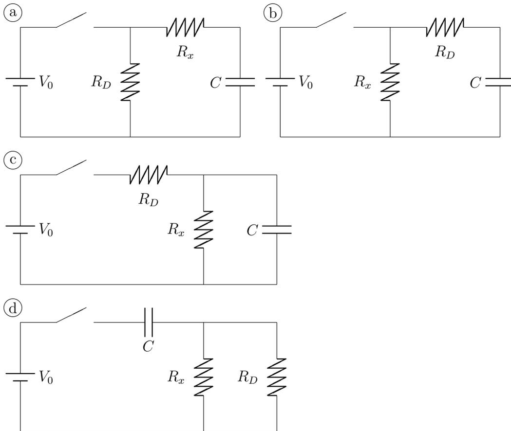
To determine which circuit will do the job, analyze all four to find  $I_D$ , the current through your device  $R_D$ . First look at their behavior at  $t = 0$ , immediately after the switch is closed, and there has been no time from charge to build up on the capacitor. Then look at their behavior at long times  $t \gg RC$ , when the capacitor has been fully charged. And then, sketch  $I_D$  vs  $t$  for all four circuits.
