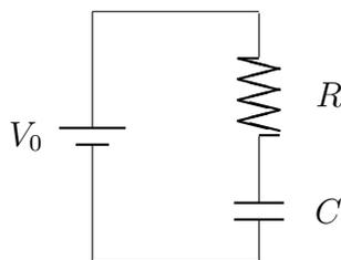
If we now quickly disconnect the voltage source, and allow the capacitor to discharge across the resistor,  $q$  will decrease—quickly at first, then more slowly—according to the relation
