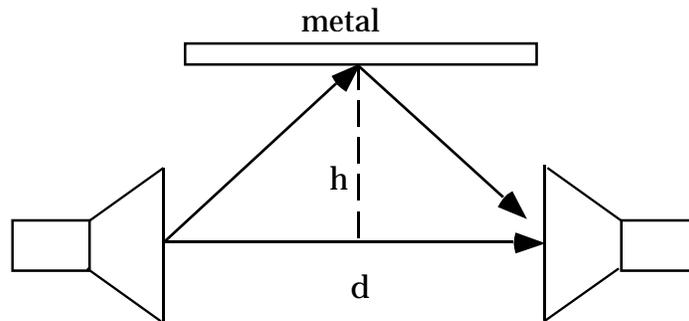
Let  $m$  be the number of wavelengths by which the two paths differ at destructive interference ( $m = 1, 2, 3, \dots$ ). Put your knowledge of geometry to use by *calculating* the height  $h$  at which you get destructive interference. That is, find  $h$  as a function of  $d$ ,  $m$  and  $\lambda$  for destructive interference.
