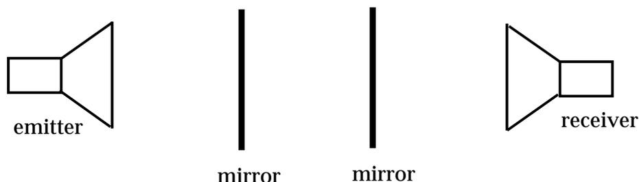
Using the set-up shown above, carefully measure the distance  $d$  you need to move one mirror for there to be 11 successive maxima (that is, 11 successive positions in which there is a strong standing wave). The distance between the first and eleventh maxima must correspond to 5 wavelengths.
