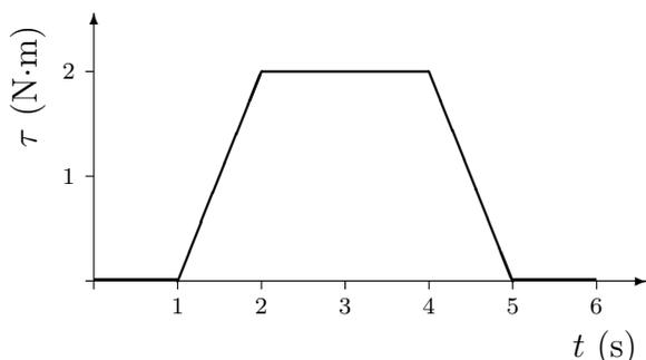
**Answer:** Just like the area under a  $F$ - $t$  curve is  $\Delta p$ , the area under this  $\tau$ - $t$  curve will be  $\Delta L$ . The area is  $\Delta L = 6 \text{ N}\cdot\text{m}\cdot\text{s}$ . At first,  $L_i = I\omega_i = 0$ . Therefore
