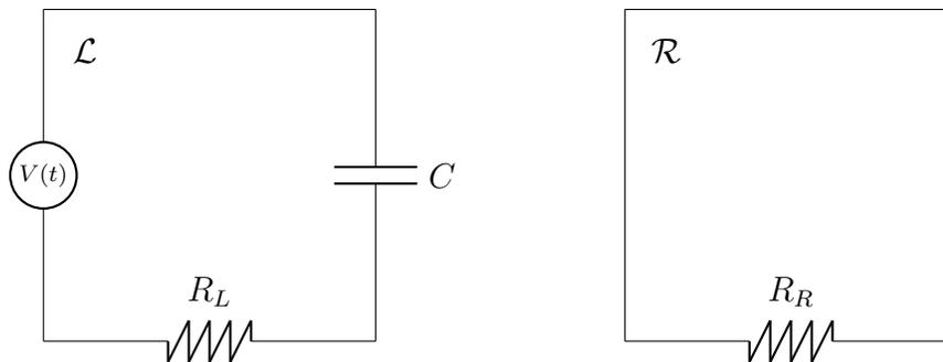
Circuit  $\mathcal{L}$  has a voltage source which is a function generator that produces a square waveform  $V(t)$ , which looks like the following on an oscilloscope:
