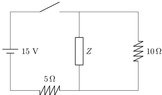
**Answer:** The junction equation:  $I_1 = I_2 + I_3$ , where  $I_1$  is the current through the battery and the  $5\ \Omega$  resistance,  $I_2$  is the current through the zingschritt, and  $I_3$  is the current through the  $10\ \Omega$  resistance.
