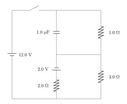
(a) Find the currents through all the resistors *immediately after* the switch is closed, before the capacitor has any time to charge up at all.
