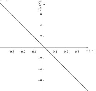
(b) The oscillations of a single spring have an angular frequency  $\omega = \sqrt{k/m}$ . What is the angular frequency for the oscillations of this double spring setup? Explain.
