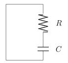
This is what you will observe on the oscilloscope as we alternately charge and discharge the capacitor. This is accomplished by using a square wave voltage, which is equivalent to attaching and disconnecting a battery: when in square wave mode, the function generator alternates between  $V = V_0$ and V = 0. The capacitor will charge when the square wave is at  $V = V_0$ , discharge when the square wave is at V = 0, charge, discharge, ...
