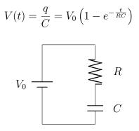
If we now quickly disconnect the voltage source, and allow the capacitor to discharge across the resistor, q will decrease—quickly at first, then more slowly—according to the relation
