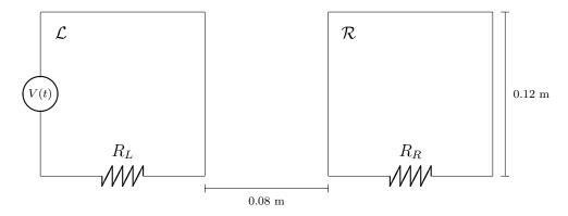
Each circuit is square with 0.12 m sides, and 0.080 m separates the right edge of the left circuit ( $\mathcal{L}$ ) from the left edge of the right circuit ( $\mathcal{R}$ ). Both have the same resistance values  $R_L = R_R = 0.50 \Omega$ , and  $\mathcal{L}$  has a voltage source which produces a sawtooth waveform V(t), which looks like the following on an oscilloscope:
