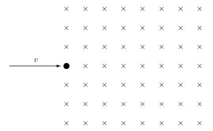
**Answer:** This magnetic field will produce a force  $F_B = evB$ , always perpendicular to the velocity. This bends the electron in a circular path. By the right-hand-rule, and the fact that the electron has a negative charge,  $\vec{F}_B$  will point downward on the page. Therefore the electron bends downward in a circular arc.
