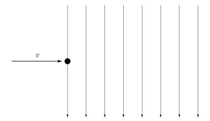
**Answer:** The electric force is  $F_E = eE$  in magnitude. Since the electron charge is negative,  $\vec{F}_E$  points upward on the page. This *constant* force will bend the electron upwards, in a parabolic trajectory.
