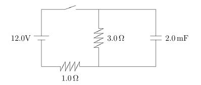
**Answer:** At t = 0, the capacitor starts charging up, and short-circuits the  $3\Omega$  resistor. We get  $I_1 = (12 \text{ V})/(1 \Omega) = 12 \text{ A}$ .
