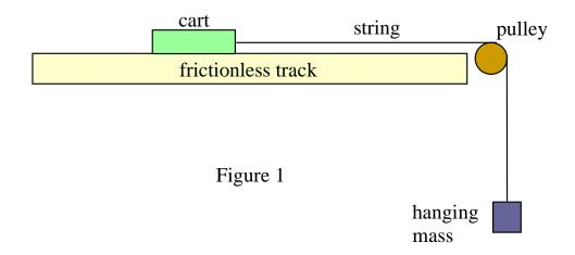
(a) **Track not frictionless:** A small extra kinetic friction force on the cart toward the left slows the cart down, increasing the measured  $\Delta t$ . The equation for g was
