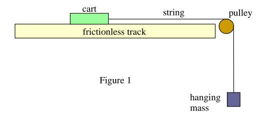
(a) **Track not frictionless:** A small extra kinetic friction force on the cart toward the left slows the cart down, increasing the measured  $\Delta t$ . The equation for g was
