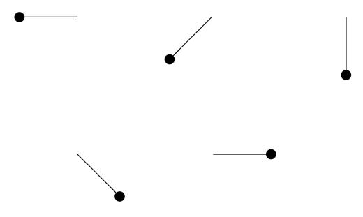
Answer: The tension in the string does not contribute to torque, since it is always directed toward the axis of rotation. So the total torque is due entirely to the weight:  $\tau = mgl \cos \theta$ .
