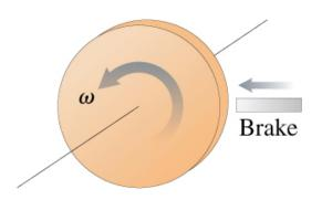
**Answer:** Use  $\Sigma \tau = I\alpha$ . Any forces on the axle will produce no torque, since their distance to the axis of rotation is zero. The normal force at the brake contact is completely parallel to the line connecting it to the axis of rotation; it has zero perpendicular component. The friction, on the other hand, is completely perpendicular to that line, and it will be the only force producing a torque.
