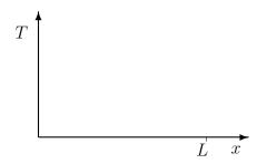
(c) You have a double-glazed window between the inside of a room at  $T_{in}$  and the outside at  $T_{out}$ . The thickness of the two glass panes and the air trapped is all equal, L. The thermal conductivity of air is less than glass:  $k_a < k_g$ . Make a graph of T(x), the temperature within the window, with x = 0 one side of the slab and x = 3L the other side. Give your reasoning for what you drew.
