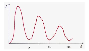
**Answer:** There are two paths for waves between the source and detector. You can see from the geometry of the experiment that the path length difference is  $l_1 - l_2 = d$ . There is also a phase shift of  $\lambda/2$  due to the reflection off the mirror. Therefore, the condition for constructive interference is  $d = (m + \frac{1}{2})\lambda$ , while destructive interference happens at  $d = m\lambda$ , where m is an integer.
