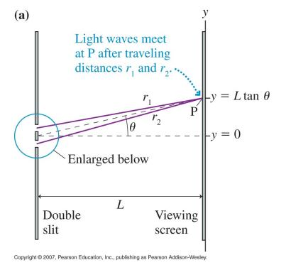
In your case, however, you will find it easier to measure the angle  $\theta$  directly, with your apparatus, rather than dealing with L and y values. Record the intensity I at various values of  $\theta$ . Make a graph of how I depends on  $\theta$ . (Don't worry about units for I, because we only care about relative intensities, not absolute values.)
