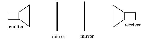
Using the set-up shown above, carefully measure the distance d you need to move one mirror for there to be 11 successive maxima (that is, 11 successive positions in which there is a strong standing wave). The distance between the first and eleventh maxima must correspond to 5 wavelengths.
