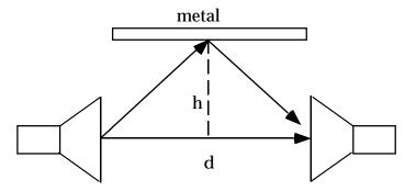
Let m be the number of wavelengths by which the two paths differ at destructive interference ( $m=1,2,3,\ldots$ ). Put your knowledge of geometry to use by calculating the height h at which you get destructive interference. That is, find h as a function of d, m and  $\lambda$  for destructive interference. (You won't need trigonometry, just the Pythagorean theorem.)
