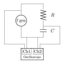
Set up the circuit shown. The oscilloscope should be set to view both traces; be sure you know which trace is which voltage: Ch1 is the function generator and Ch2 is the capacitor. Set the function generator to square wave, about 1000 Hz, and any voltage greater than zero. The R shown in the diagram is actually a series combination of the external resistance (the decade resistance box) and the internal resistance of the function generator
