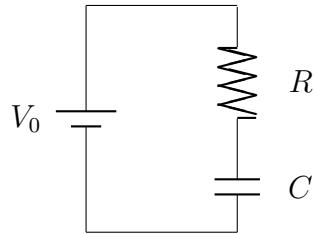
If left for long enough, the charge on the capacitor will increase from  $q = 0$  to  $q = CV_0$ . During that time,  $q$  will change with time according to the relation
