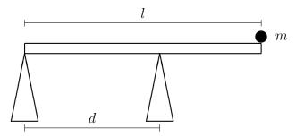
Answer: The center of mass of the plank is at its middle, a distance of l/2 from the left end. If nothing is moving, two equations must be satisfied:  $\sum F_y = 0$  and  $\sum \tau = 0$ . Take the axis of rotation to be at the left end at the plank. (It doesn't matter where you choose the axis to be.) The normal force applied by the small mass on the plank is downward and is mg in magnitude.
